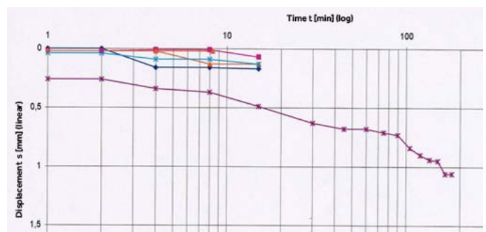
Suitability test: Determination of creep values
