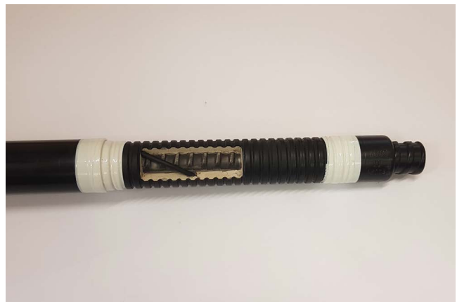
Example of a Double Corrosion Protection System (DCP)
